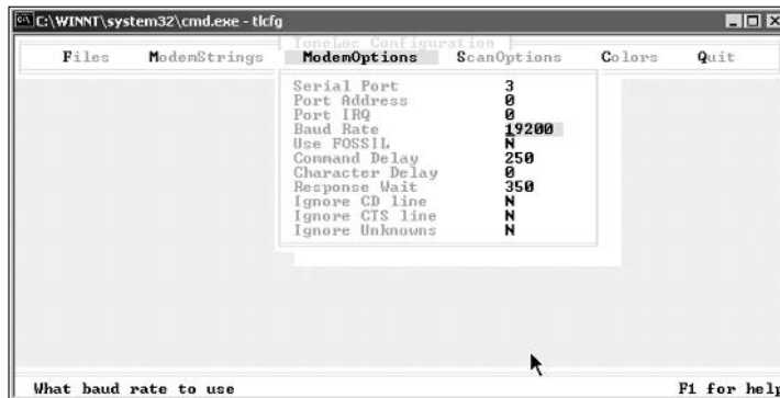
Figure 8-1: Configuring the modem in ToneLoc's TLCFG utility.
